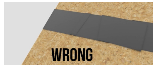
Figure 4. Right and wrong installation of tape over seams.
