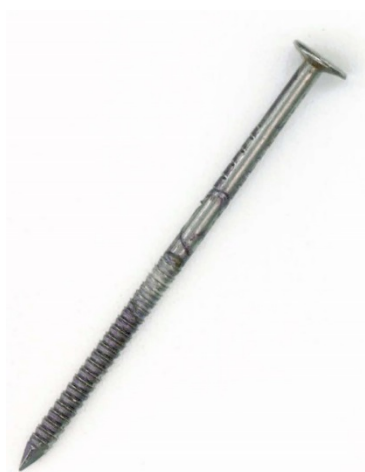
Figure 2-10. Use 8d ring-shank nails as the added fasteners when re-nailing roof sheathing. Research indicates that ring-shank nails have about twice the uplift capacity of the same size smooth-shank nails.
