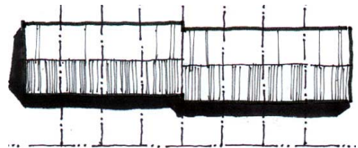
Figure 3-1. Townhouse units of more than 4 shall have a differentiated front building line of at least 4 feet and no single building shall have more than 8 units.
